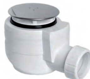
Scarico doccia in ABS 90 x 40 ECO tappo ø 115 cromato uscita acqua 45 l/min Shower tray waste ABS ECO 90 x 40 with ø 115 chrome plated cover water flow 45 l/min
